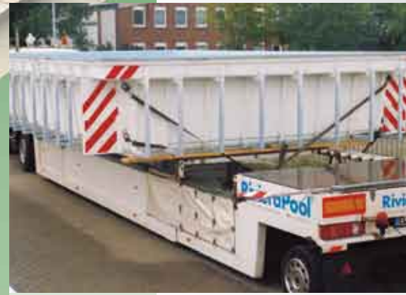
Oversized pools: Prefabricated pool with overflow channel and steel supports fixed to the pool.
