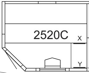
Screw the 350 mm batten (marked X) onto the lower bench and the batten marked Y onto the wall. Fit the armrest (2025/2025C).
