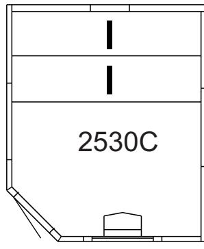
Screw the bench support battens to the rear of the left and right-hand walls, as shown. Then put the prefabricated rear sauna benches in place and add the centre support.
